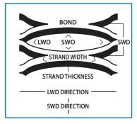
STRAND THICKNESS - Gauge thickness of the base metal.
